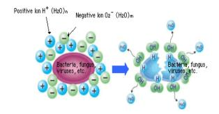
Mechanism for Inactivating Bacteria, Fungi
